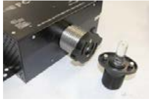
6) Reattach existing fiber port to new unit
