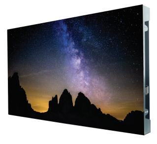
The **PXL-FX1.56-E** Video Cabinet by Impact Lighting delivers superb image quality with a 1.56 pitch RGB display that features an IP45 ingress rated Aluminum and Magnesium Alloy Cabinet, providing serviceability from the front and back. Each cabinet is 0.2025 sq. meters. Overall dimension of each cabinet is 337.5mm x 600mm x 80mm (13.28" x 23.6" x 3.15")
