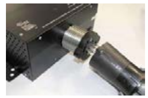
2) Re-attach fiber harness to new unit
