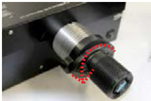
9) Twist fiber port counter clockwise until tight
