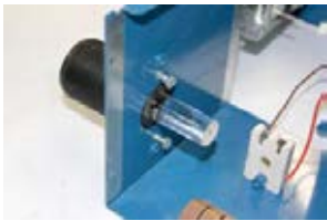
3) Remove 2 screws inside unit securing fiber port
