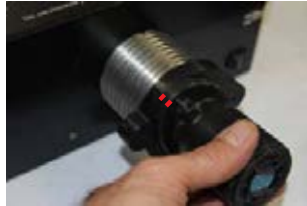
8) Align screw heads with slotted holes
