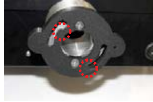
7) Locate slotted holes on new fiber port
